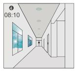
When natural light levels exceed setpoint off to light, the light will turn off even if the space is occupied.
