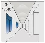
The light automatically turns on at 10% when natural light is insufficient (no
