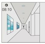
When natural light levels exceed setpoint off to light, the light will turn off even if the space is occupied.
